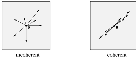
Fig. 1.8 When restricted to a small block of lattice points, the O(V) low modes of the Dirac operator tend to align to a relatively low-dimensional linear space, a property referred to as local coherence.
